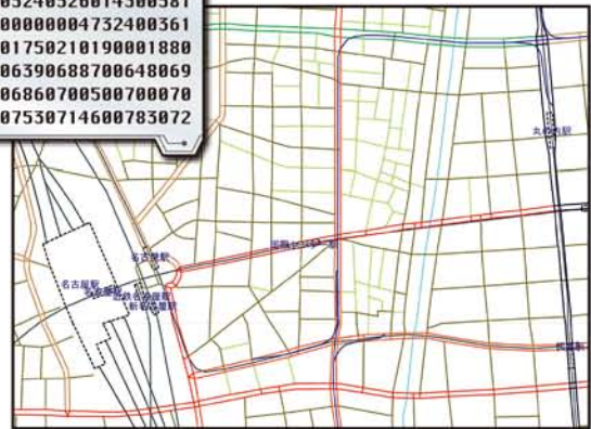
Digital Road Map (The digital road is recorded as a set of numbers and letters. This is an example of a depicted image produced by software that can convert this alphanumeric data into visual form.)
