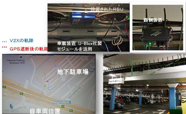
写真13 GPSless Positioning for V2X(Cohda Wireless社)
