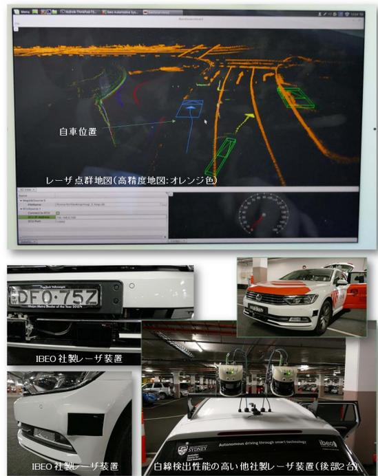
写真14 Real-time localization and reference generation in urban traffic (Ibeo Automotive Systems GmbH社)
